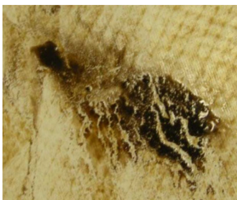
Fig. 10. Deposit of MnO_2 on RO membrane
