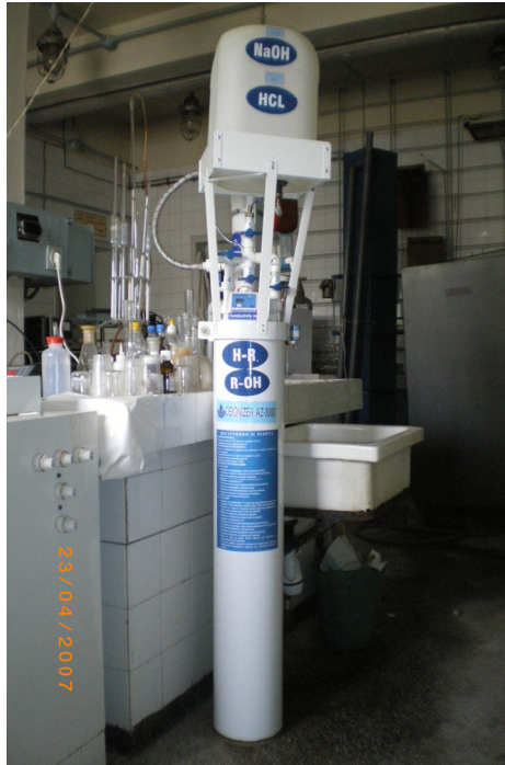
Fig. 8. Photography of a pilot one body multi stage multi cell water deionization filtration device
