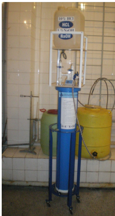
Fig. 13. Photography of a multi process ion-exchange and sorption small water conditioning device (Zvezdov A.,1997; Zvezdov A.,1999; Zvezdov A., et al.2006)
