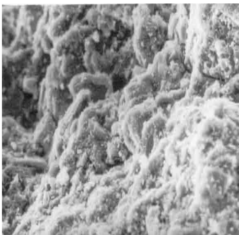
Fig. 5. Electron scanning microphotography of weak base anion-exchange Dowex MWA-1 (magnified 10 4 times)
